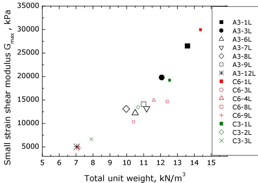
Figure 2. Small-strain shear modulus vs. total unit weight for a confining stress of 75 kPa.
