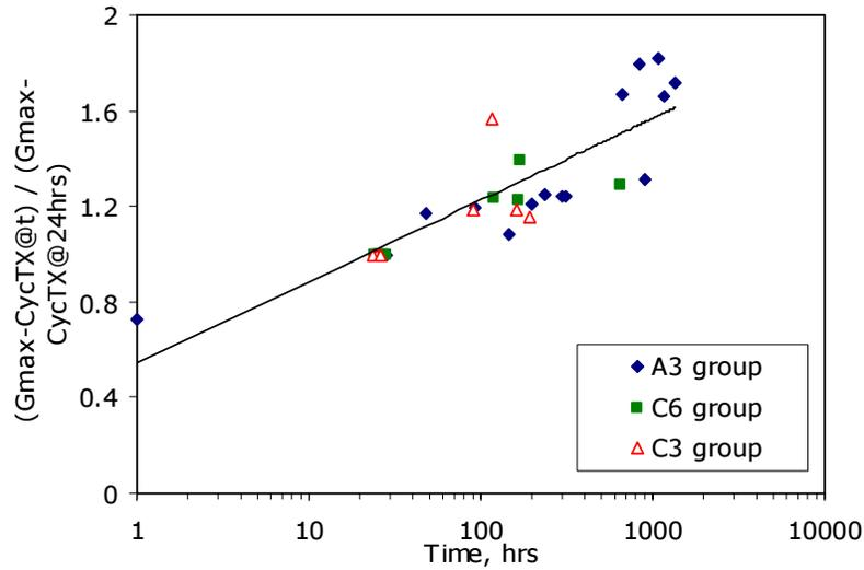
Figure 3. Change of small-strain shear modulus as a function of time under confinement.
