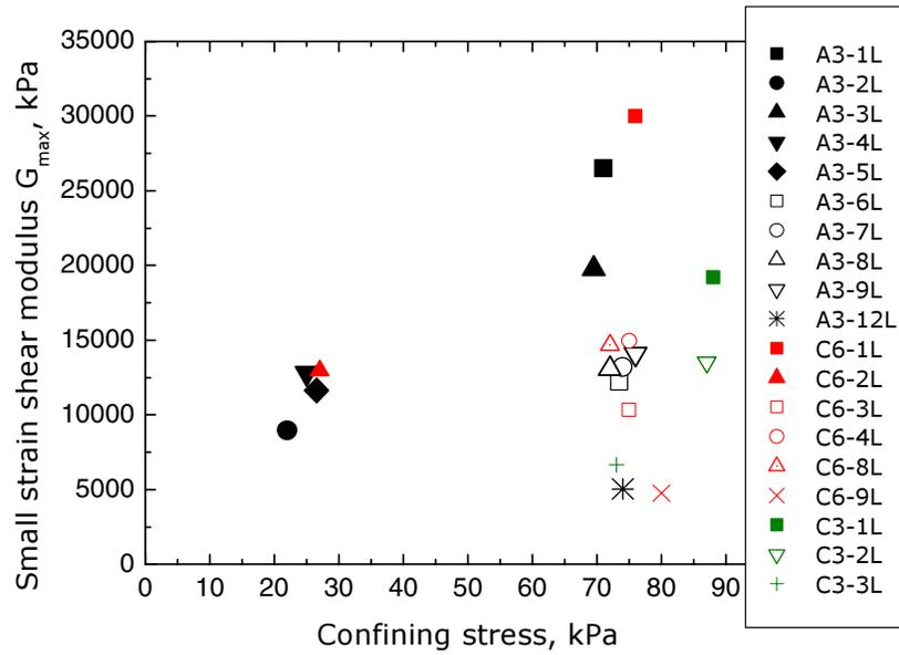
Figure 1.  $G_{max}$  vs. confining stress for MSW specimens
