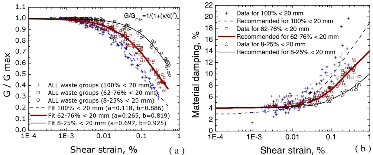
Figure 5. Results of cyclic triaxial tests from all sample groups: a) normalized shear modulus reduction curve, and b) material damping curve as a function of shear strain.
