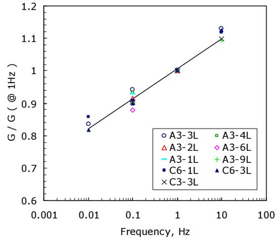
Figure 4. Effect of loading frequency on the shear modulus.
