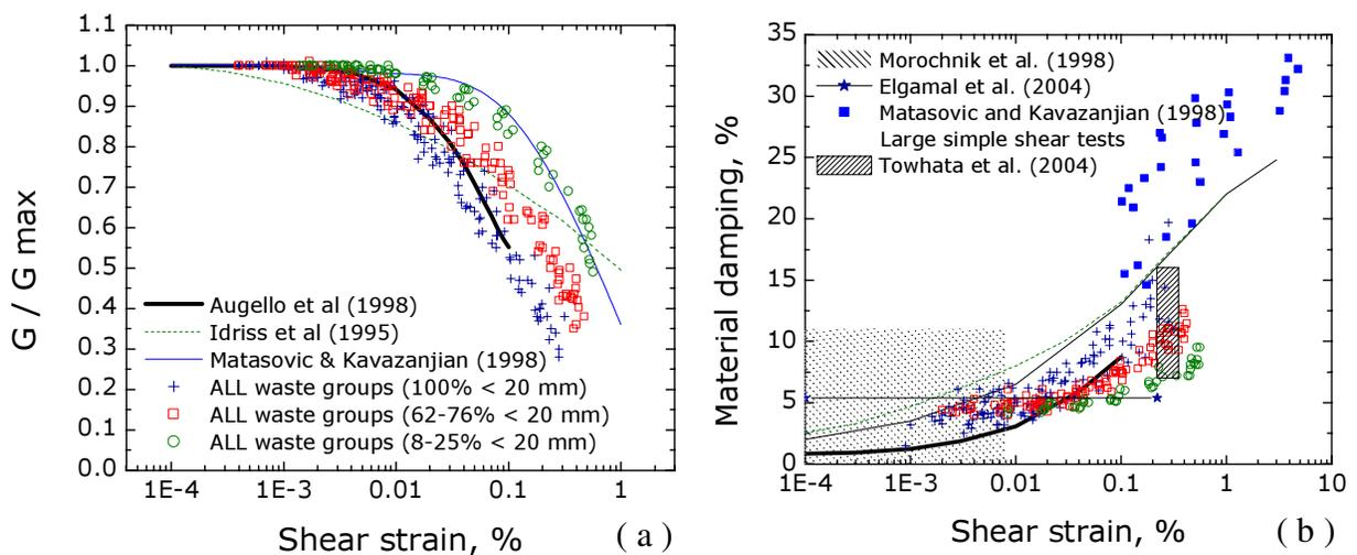
Figure 6. Cyclic triaxial test results and comparison with the literature: a) Normalized shear modulus reduction curve, b) Material damping curve, as a function of shear strain.
